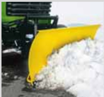
Blade For material handling, this blade does a great job – in summer and winter. • 137 cm (54 in) • 27° angling
