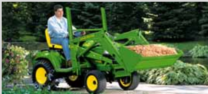
45 Loader • Installation in 5 minutes or less, no tools required • Provides required down pressure for digging action • Huge 1.22 m (48 in) bucket with 140 ltr (5 cu ft) capacity • Breakout force: 501 kg (1105 lbs); Lift height: 1854 cm (730 in)
